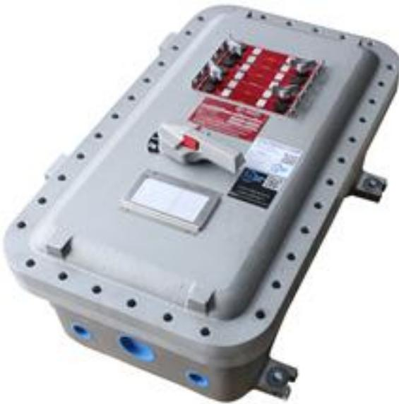
The EPPB-3P4W-3X20A.1P-1X15A.1P-1X20A.2P is an explosion proof lighting panelboard that is designed for Class I, Divisions 1 & 2 and Class II, Divisions 1 & 2 industrial facilities. This panelboard is rated at 120/240V single phase, has a 3-pole 4-wire configuration and features a 100-amp main breaker rating with three, 20-amp single phase; one, 15-amp single phase; and one, 20-amp two phase branch breakers.
